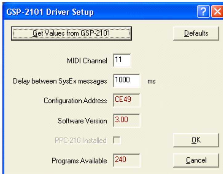
When you power on the GSP-2101, it automatically sends a couple of MIDI messages that we use to get started. After these, we exchange other MIDI messages that let us know things like which EPROM (chip-set) version is installed, whether or not an optional PPC-210 co-processor board is installed, and how many user and factory programs are available.
